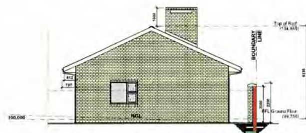
NORTH EAST ELEVATION (SINGLE STOREY) scale 1:100
