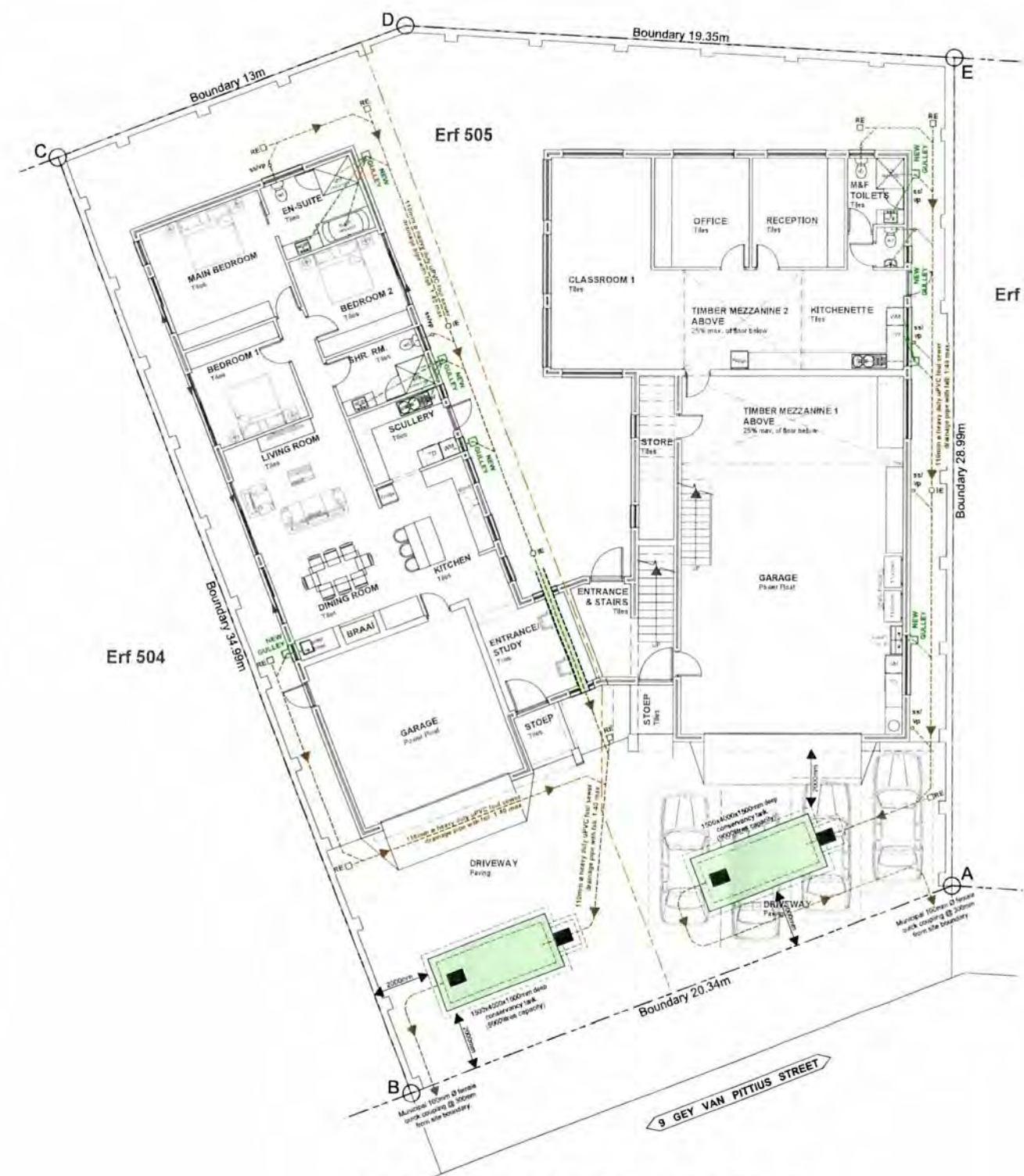
GROUND FLOOR DRAINAGE PLAN scale 1:100
