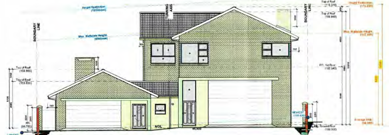
SOUTH WEST ELEVATION scale 1:100
