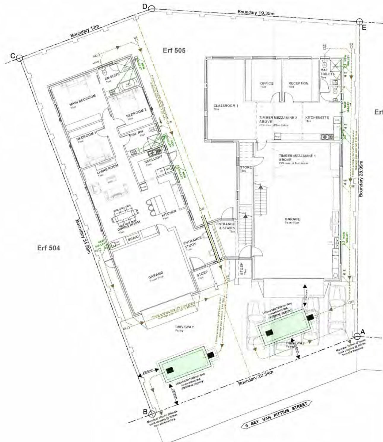
GROUND FLOOR DRAINAGE PLAN scale 1:100
